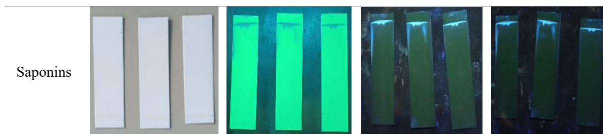
Figure 1. KLT results of secondary metabolite compounds. The results were observed in (a) visible light (b) UV light 254 nm (c) UV light 366 nm (d) UV light 366 nm after being sprayed with color reagent
